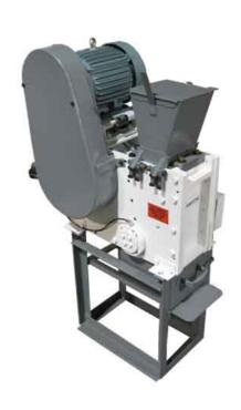
New opening adjustment on one side only is fool proof and achievable with only two screws! Customers' feedback and experience gave us the means to change crushing drive components to the point where this machine will outlast previous models and comparable competitor's machines for a long time!
